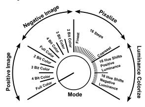
**Control Voltages** - All five of the controls on the MVIP have coresponding control voltage inputs, and each of those have an attenuator. So oscillators or other CV sources can be used to adjust the brightness or hue controls, sweep through the various bitswap modes, or change the main mode function.
