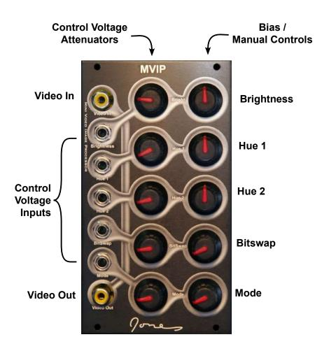
**Brightness** - Controls the brightness of the incoming video. When using the bitswap feature, the brightness control pushes the incoming video up and down through the various thresholds created by the bitswap. Otherwise it simply lightens or darkens the video.
